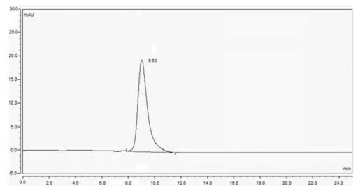
Aggregate analysis by SEC-HPLC of non-PEGylated Fab'
